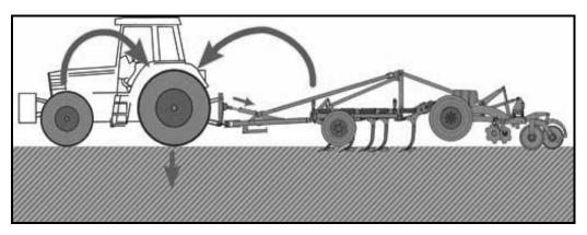
5.1.1 Describe TWO ways in which the mass displacement of a tractor can be positively influenced.
