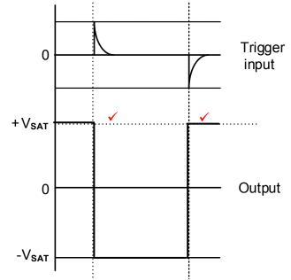
NOTE  $R_1$  acts as a pull down resistor ensuring that during switch on, the output will start at  $+V_{SAT}$
