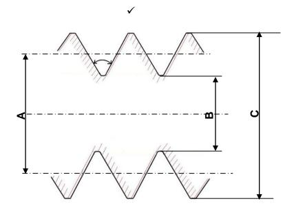
A = Pitch diameter/Effective diameter  $\checkmark$
