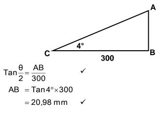
$$d = D - 2(AB) \qquad \checkmark = 200 - 2(20,98) \qquad \checkmark = 158,04 \text{ mm} \qquad \checkmark$$
