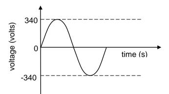
10.2.1 Write down the maximum (peak) output voltage of the generator. (1)
