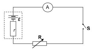
The learners use their recorded readings of current and resistance, together with the equation R =  $\frac{\epsilon}{r}$  – r, to obtain the graph below.
