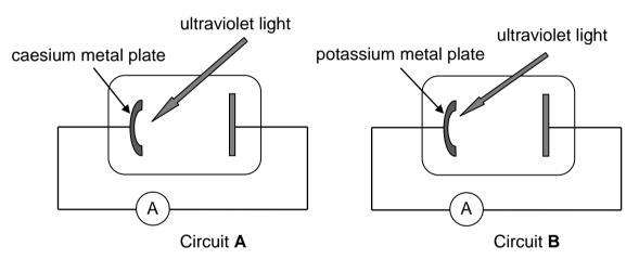
Ultraviolet light with the same intensity and wavelength of 5,5 x  $10^{-7}$  m is incident on the metal plate in EACH of the photocells and the ammeter in circuit **A** registers a current.
