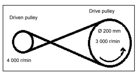
5.5.1 Calculate the diameter of the driven pulley by using the following formula:
