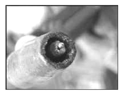
4.1.1 A farm worker was repairing an implement with the aid of a MIG welding machine. Suddenly the wire fused itself to the welding tip.
