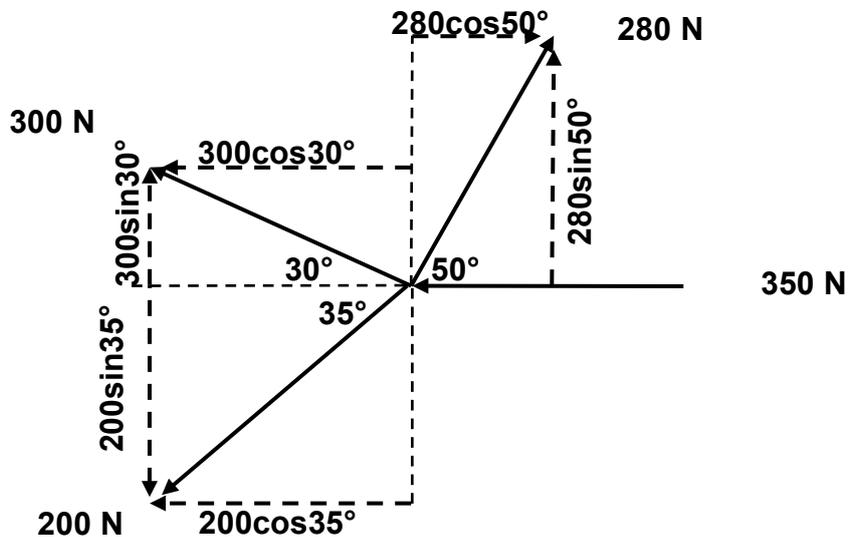
$$\begin{aligned} \sum HK &= 280\cos 50^\circ - 200\cos 35^\circ - 300\cos 30^\circ - 350 \\ &= 179,98 - 163,83 - 259,81 - 350 \\ &= -593,66\text{ N} \end{aligned}$$
