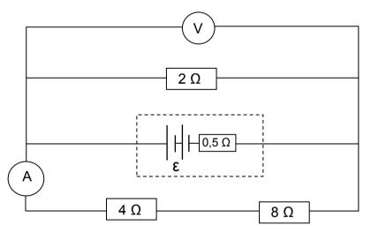
The reading on the ammeter is 0,2 A.
