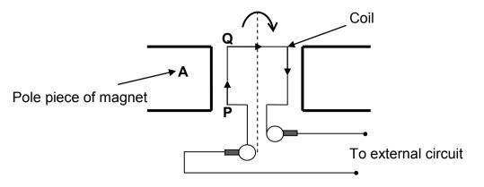
The coil of the generator rotates clockwise between the pole pieces of two magnets. At a particular instant, the current in the segment PQ has the direction shown above.
