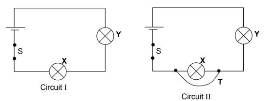
A wire **T**, of negligible resistance, is now connected across **X** as shown in Circuit II.
