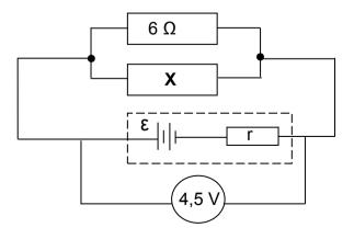
9.2.3 Calculate the resistance of **X** when the voltmeter reads 4,5 V.
