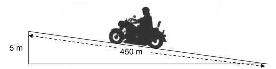
The total frictional force acting on the motorbike is 294 N. The combined mass of rider and motorbike is 300 kg. The average driving force on the motorbike as it moves up the incline is 350 N. Consider the motorbike and rider as a single system.
