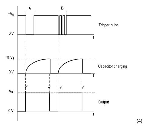
4.4.2 Trigger pulse B looks like a series of 'on' and 'off' pulses. ✓ This is known as switch bounce. ✓(2)
