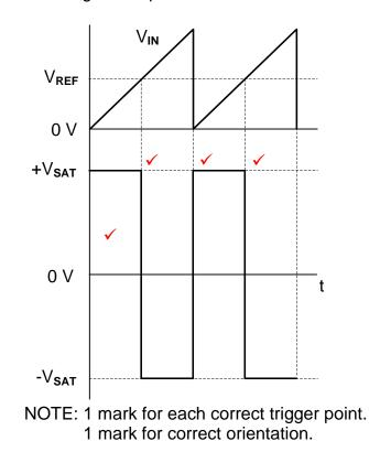
2.6.3 The op-amp is used in open loop mode therefore; ✓ there is no feedback loop to limit the gain of the op-amp, ✓ driving it into saturation.
