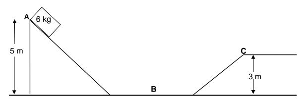
5.2.1 State the principle of conservation of mechanical energy in words. (2) 5.2.2 Calculate the mechanical energy of the block at point **A**. (4) 5.2.3 What will be the speed of the block at point B? (4) 5.2.4 Calculate the speed of the block at point **C**. (4)
