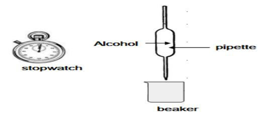
The learners use a stopwatch to measure the time it takes a FIXED VOLUME of each of the alcohols to flow from the pipette. They record this flow time, which is an indication of the viscosity of each alcohol, as given in the table below.
