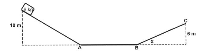
The frictional force between the surface and the block is 20 N as it moves from B to C.
