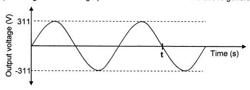
The output voltage is generated at a frequency of 50 Hz.
