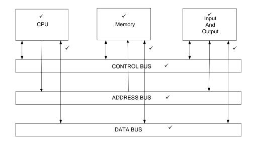
6.4.2 A shared boundary ✓ across which two separate components of a computer system exchanges information. ✓
