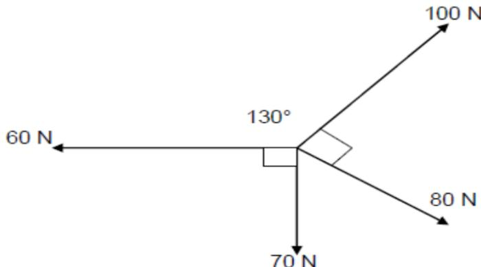
$$\begin{aligned} X_{\text{kom}} &= 100 \cos 50 + 80 \cos 40 - 60 & \checkmark \\ &= 65,56 \text{ N} & \checkmark \end{aligned} \quad (2)$$
