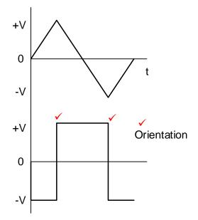
NOTE: 2 The trigger points are only accepted if the wave shape is correct.
