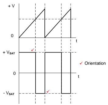
**NOTE:** 1 mark for orientation 1 mark for each correct trigger point
