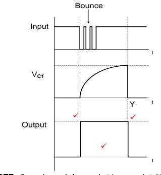
**NOTE:** 2 marks = 1 for each trigger point (the output must be a square wave)
