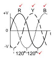
**NOTE:** The sequence of R,Y,B ( $V_{L1}$ ,  $V_{L2}$ ,  $V_{L3}$ ) must be correct to be awarded full marks
