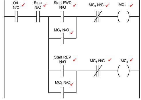
**NOTE:** O/L and Stop must both be in the same condition (either open or closed)
