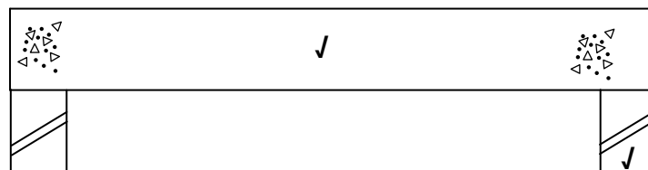
Simple supported slab
