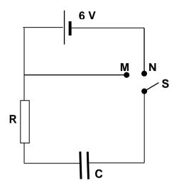
Switch **S** is initially at position N. After a while it is moved to position M.
