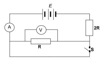
When switch **S** is closed, the reading on voltmeter V, in volts, is ...
