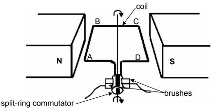
When the motor is functioning, the coil rotates in a clockwise direction, as shown.
