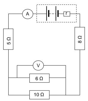
The current passing through the 10  $\Omega$  resistor is 0,6 A.
