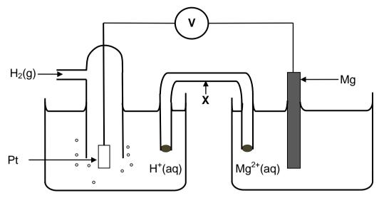
The reading on the voltmeter is 2,36 V.
