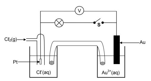
With switch **S** OPEN, the initial reading on the voltmeter is 0,14 V.
