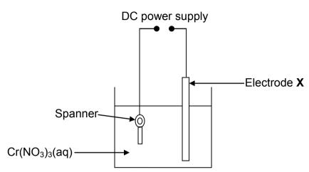
A constant current passes through the solution and the concentration of  $Cr(NO_3)_3(aq)$  remains constant during the process. In the process, a total of 0,03 moles of electrons is transferred in the electrolytic cell.
