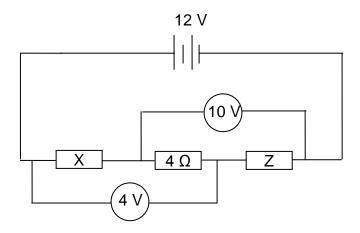
The battery has no internal resistance and the resistance of the conducting wires can be ignored.
