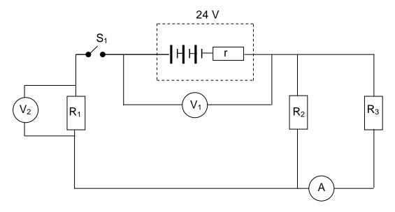
The resistance of  $R_1$  is 1,5  $\Omega$ , the resistance of  $R_2$  is 10  $\Omega$ , while the resistance of  $R_3$  is unknown.
