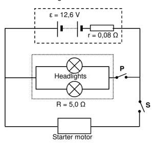
8.2.1 Write down the magnitude of the potential difference across switch **S** when both switches are open.
