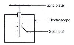
When the zinc plate is irradiated with visible light, no change is observed. When the zinc plate is irradiated with ultra violet light, the gold leaf falls back.
