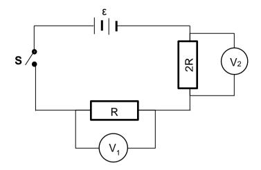
When switch **S** is closed, the reading on voltmeter  $V_1$  is  $\frac{1}{3}\epsilon$  and the reading on voltmeter  $V_2$  is ...
