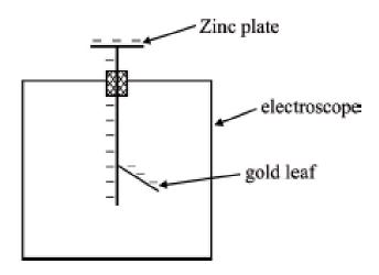
When the plate is irradiated with visible light, nothing is observed. When the plate is irradiated with ultraviolet light the gold leaf collapses.
