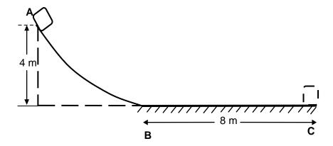
An object of mass 10 kg is released from point **A** which is 4 m above the ground. It slides down the track and comes to rest at point **C**. Which ONE of the following statements about the mechanical energy of the 10 kg mass is CORRECT if it loses energy along BC?
