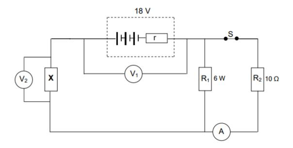
When switch **S** is **closed**, the ammeter **A**, reads 1,2 A while voltmeter **V**<sub>2</sub> reads 3,8 V.
