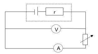
The resistance of the variable resistor is decreased. Which ONE of the following combinations of changes will occur in the ammeter and voltmeter readings?
