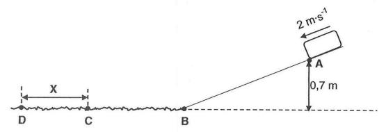
5.1 Use the LAW OF CONSERVATION OF MECHANICAL ENERGY to calculate the speed of the block at point **B**.
