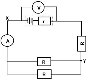
A conducting wire of negligible resistance is now connected into the circuit across points X and Y. Which combinations below correctly shows the changes to the readings on the voltmeter and ammeter?
