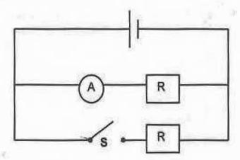
When switch S is open, the reading of the ammeter is I.
