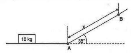
The block reaches point A at a speed of 8,84 m□s<sup>-1</sup>. It slides up the incline and comes to REST at point B after covering on distance x. A constant frictional force of 45 N acts on the block as it moves from A to B.
