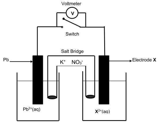
When the cell is in operation, electrons flow through the Pb electrode towards the **X** electrode in the external circuit.
