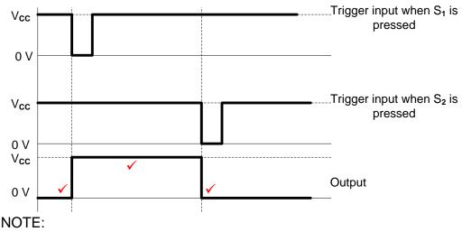
An inverted output waveform the candidate will lose 1 mark for orientation and be awarded 2 marks for the correct trigger points. (3)
