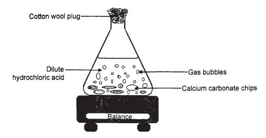
The cotton wool plug placed in the mouth of the flask prevents spillage of reactants and products, while simultaneously allowing the formed gas to escape. The balanced equation for the reaction that takes place is:
