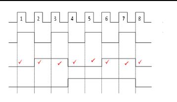
NOTE: A mark is allocated for the correct count at each clock pulse e.g. the count at clock pulse 3 should be 011 and at clock pulse 8 the count should be 000.
