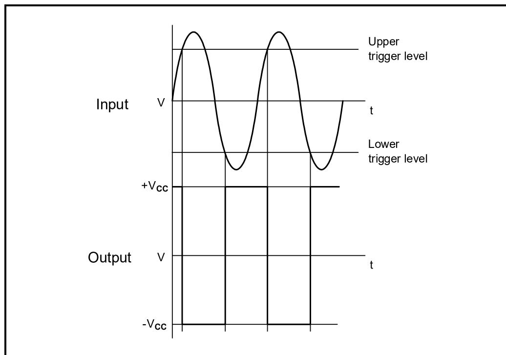
**FIGURE 3.4: SCHMITT TRIGGER INPUT AND OUTPUT**
