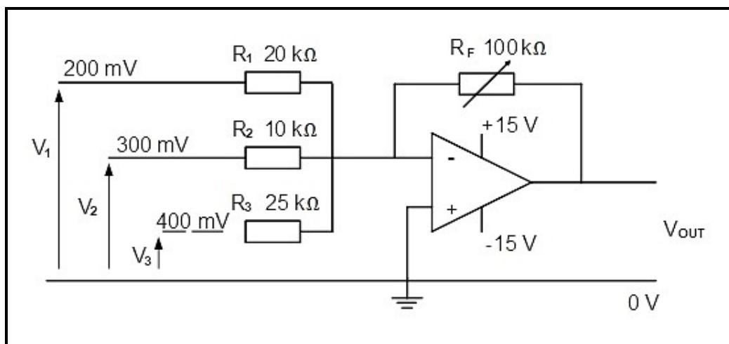
**FIGURE 3.5: INVERTING SUMMING AMPLIFIER**
