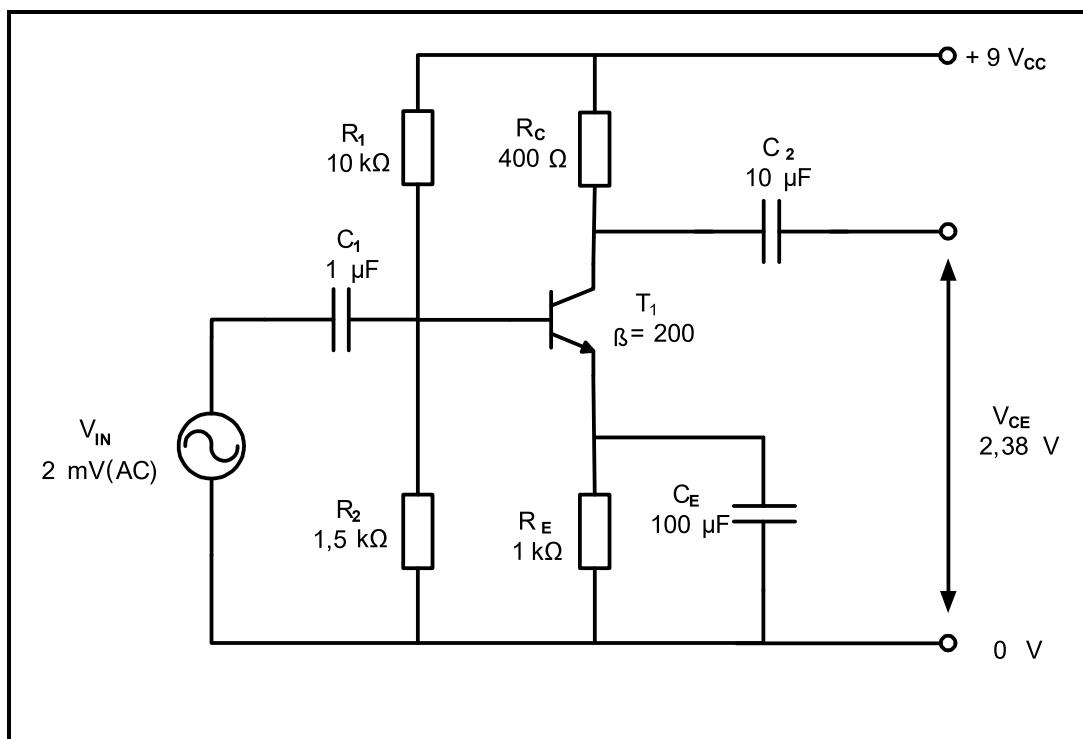
FIGURE 6.2: AMPLIFIER CIRCUIT DIAGRAM
