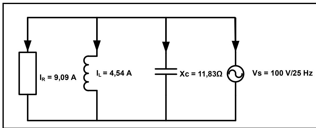
**FIGURE 3.5: PARALLEL RLC CIRCUIT**
