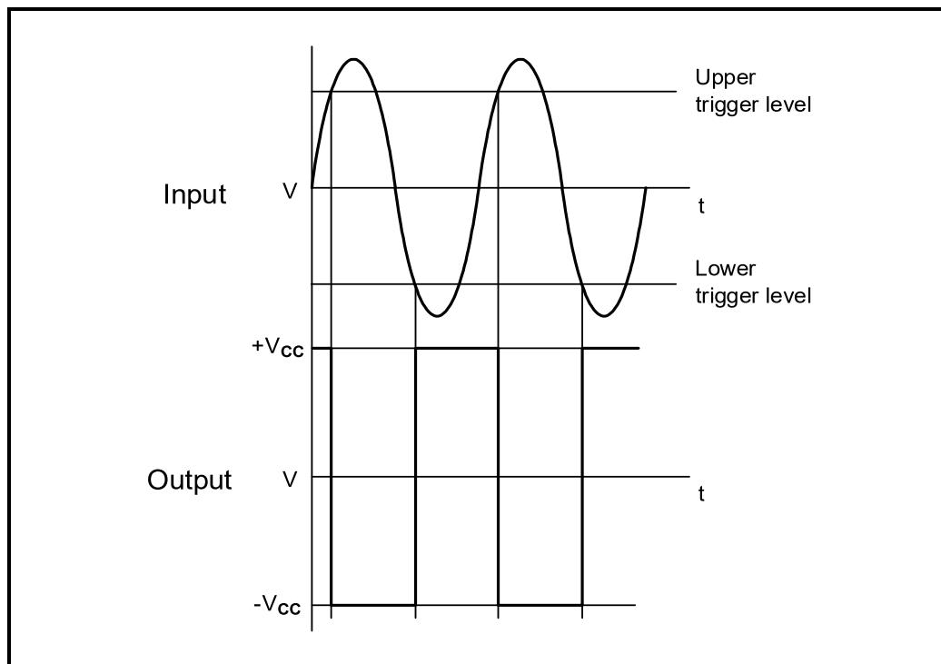
**FIGURE 5.4: SCHMITT TRIGGER INPUT AND OUTPUT**
