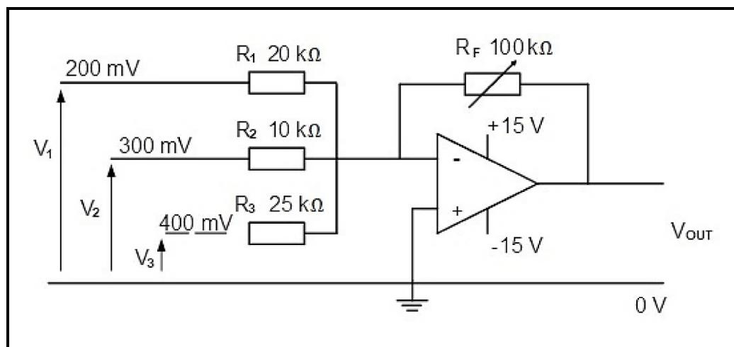
**FIGURE 5.5: INVERTING SUMMING AMPLIFIER**
