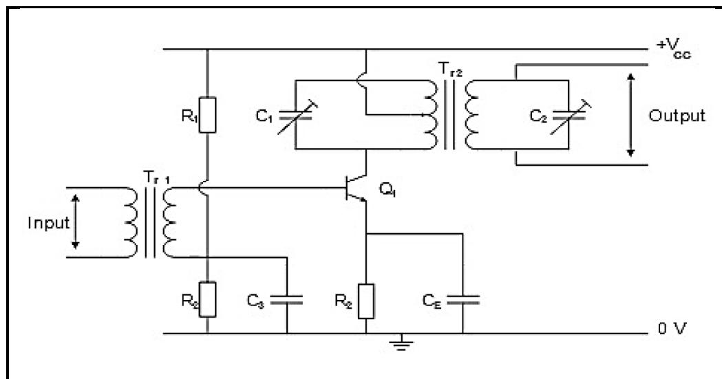
FIGURE 6.6: RADIO-FREQUENCY AMPLIFIER
