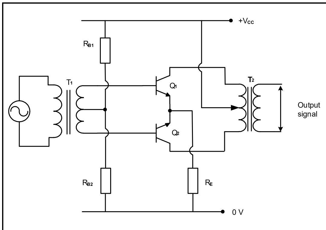
**FIGURE 6.3: AMPLIFIER CIRCUIT DIAGRAM**
