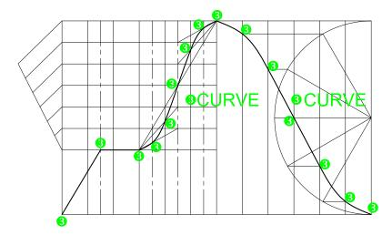
DISPLACEMENT GRAPH ✓ SCALE 30° = 8 mm
