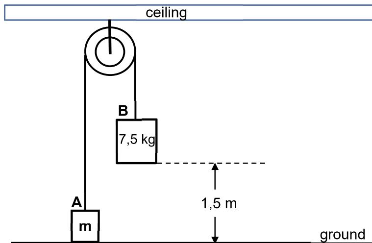
When block **B** is released, it moves vertically downwards and strikes the ground with a velocity of  $3,41 \text{ m}\cdot\text{s}^{-1}$ .
