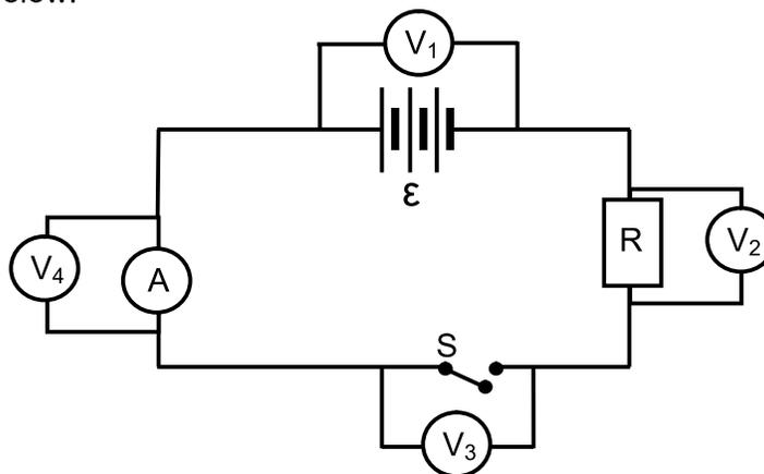
Which voltmeter(s) will have the same reading as voltmeter  $V_1$  when the switch is open?
