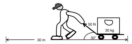
The trolley experiences a frictional force of 15 N and the bag is transported over a distance of 30 m from the loading zone to the aircraft.
