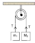
The system has acceleration "a", with  $m_2$  going down and  $m_1$  going up. This acceleration can be determined experimentally. The tension in the cord is T when the system moves.
