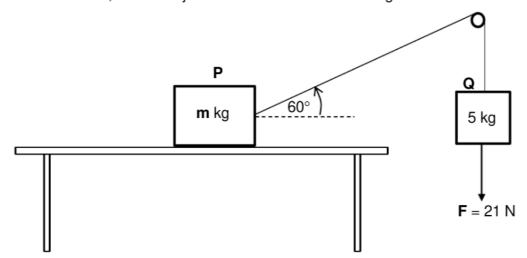
The coefficient of STATIC FRICTION between the surface of the table and object, **P**, is 0,25.
