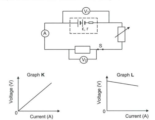
Which ONE of the combinations below CORRECTLY indicates the voltmeter readings taken to obtain graphs **K** and **L**?
