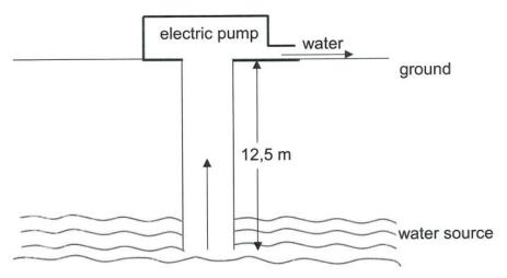
The pump lifts the water upwards at a rate of 2,5 kg·s<sup>-1</sup>. Ignore ALL frictional and capillarity effects.
