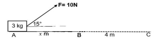
Path **AB** is x m and is frictionless and path **BC** is 4 m and is rough. The coefficient of kinetic friction between the block and the surface **BC** is 0,53. The block comes to rest at point **C**.
